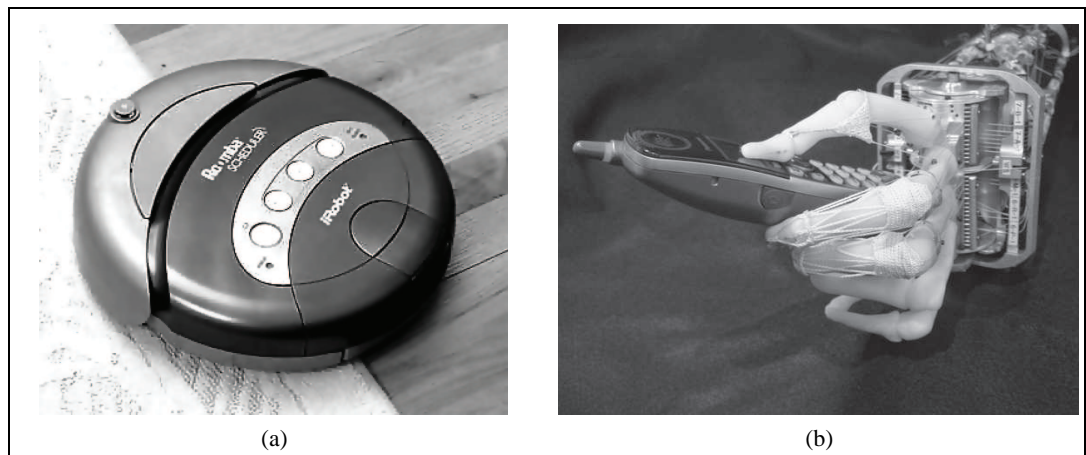
Figure 25.30 FILES: figures/roomba1.eps (Wed Nov 4 15:22:23 2009) figures/icra-cordless-phone-gray3.eps (not found). (a) Roomba, the world's best-selling mobile robot, vacuums floors. Image courtesy of iRobot, © 2009. (b) Robotic hand modeled after human hand. Image courtesy of University of Washington and Carnegie Mellon University.
