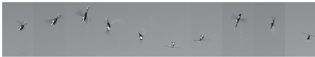
Figure 25.25 FILES: figures/flip-mosaic.eps (not found). Multiple exposures of an RC helicopter executing a flip based on a policy learned with reinforcement learning. Images courtesy of Andrew Ng, Stanford University.
