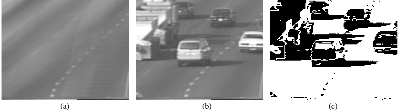
Figure 1: (a) Background image computed during fast-moving traffic using exponential forgetting. (b) Current image (frame 100). (c) Thresholded difference image showing pixels associated with moving objects.
