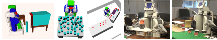
Fig. 5: Test domains from L to R: drawer domain, cluttered table with 40 objects where the dark object denotes the target object, and dinner layout. The rightmost images show the PR2 using the tray and completing the dinner layout.
